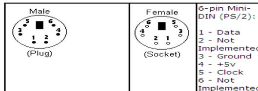
Fig.3 Pin diagram of PS2 key board
