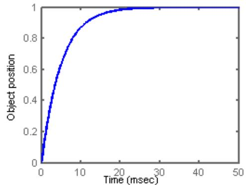
Fig. 5. Normal eye response to unit step function
