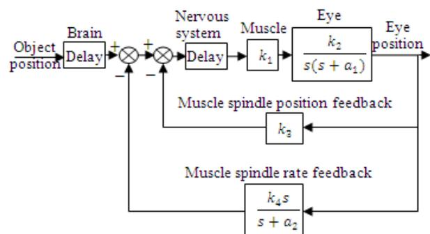
Fig. 1. Block diagram of eye movement
