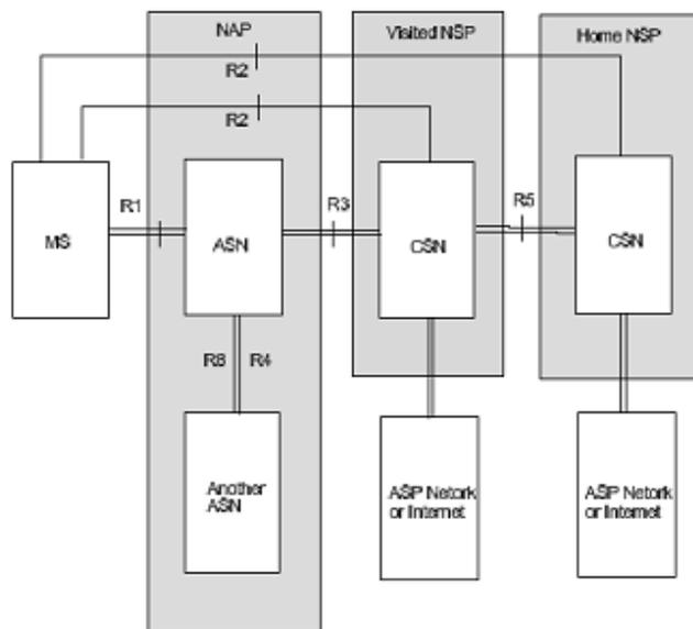
Fig 1. The WiMAX Network Reference Model
