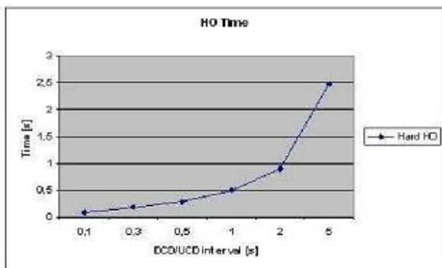
Fig 4. Measured Handover Times (Varying UCD)
