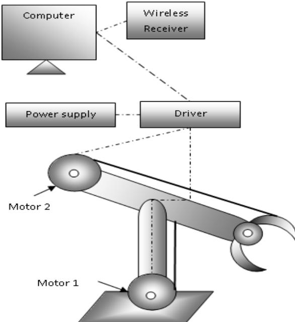
Fig. 4 Schematic diagram of the robotic arm
