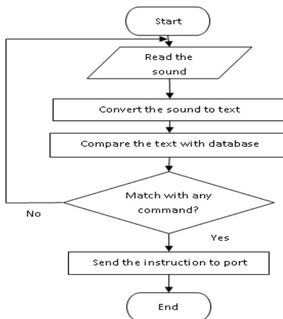
Fig. 2 Flow diagram of the robot controlling program.
