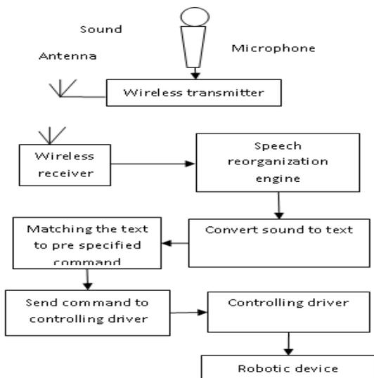
Fig. 1 Block diagram of speech recognise based robotic system
