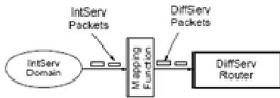
Fig. 4 Mapping function for integrated service over differentiated service.
