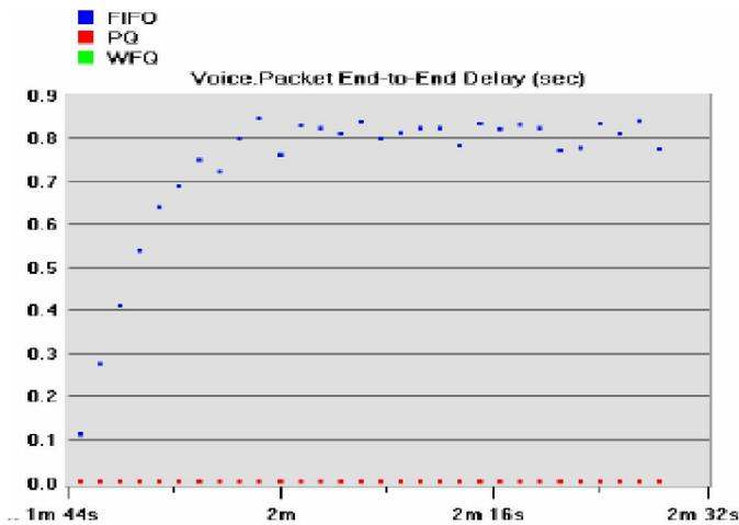
Fig. 5.4 Graphs for Voice Packet End-to-End Delay
