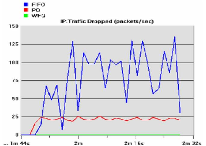
Fig. 5.1 IP packet drops (packets/sec)
