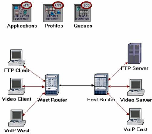
Fig. 5 Network with three different applications Procedure
