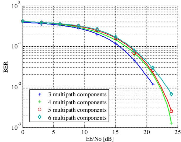
Fig. 10. BER performance of 3-RAKE receiver in multipath channel (including up to 6 multiple paths)
