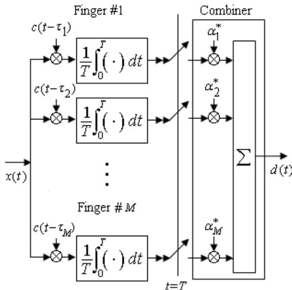
Fig. 2. RAKE receiver structure
