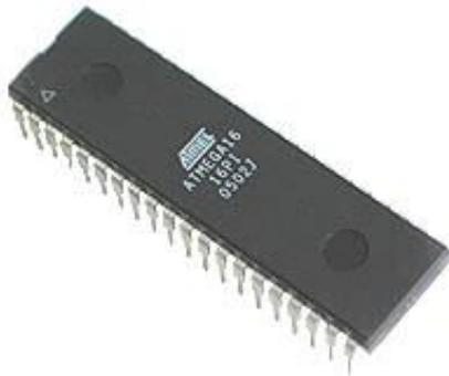
Fig. 4. Atmega 16 Microcontroller
