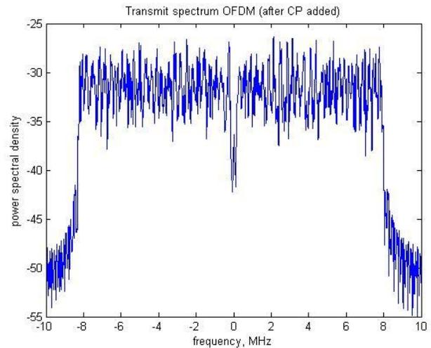
Fig. 2. Spectrum of OFDM symbol after CP added
