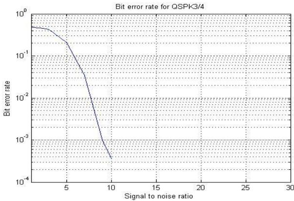
Fig. 3. Typical BER vs. Eb/N0 plot of 20 OFDM symbols transmitted
