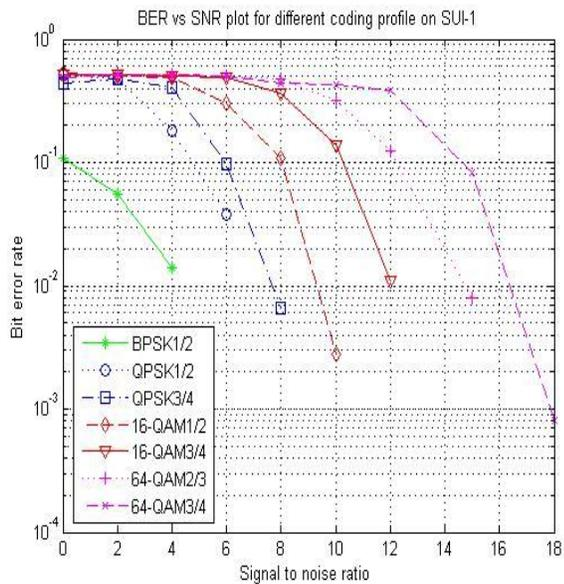
Fig. 4 . BER vs. SNR plot for different coding profiles on SUI-1 channel
